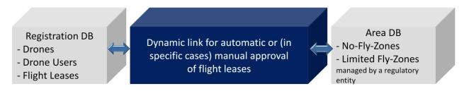
The platform enables drone users to verify where and when they can fly. On top of that, the release and referencing of a flight by the system (done automatically for the easiest cases) or its rejection, adds to the safety of any drone flying operation. The system also provides authorities with the possibility to track and verify the authorization of a drone while in operation.
